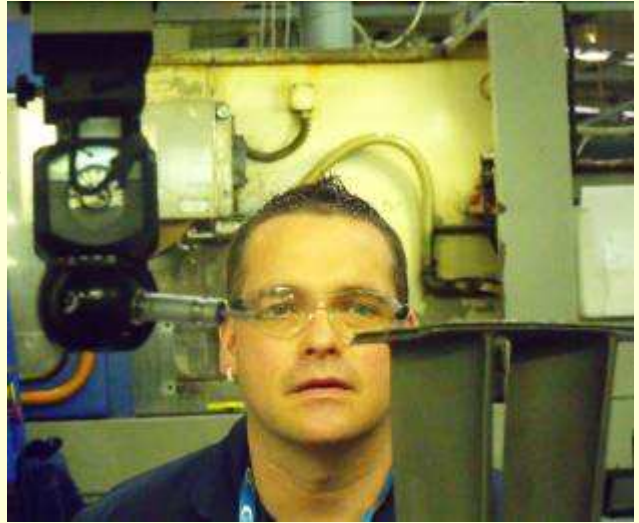
Johnathan Hemstock uses the CMM to inspect a Trent LP Blade Turbine Seal Fin.
